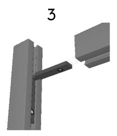
Insert the shelf's profile into the fixed angle
